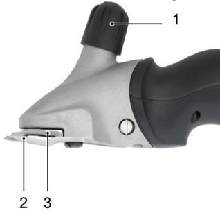
The clipper is used for clipping cattle and horses. Two comb-shaped blades are the cutting tool. The lower blade (2), which is closest to the animal's skin, is fixed and attached to the housing. The top blade (3) is agitated crossways that one. The upper blade is set in motion with the help of a pivot lever. The clipping pressure between the blades is adjusted via the adjustable head (1).
